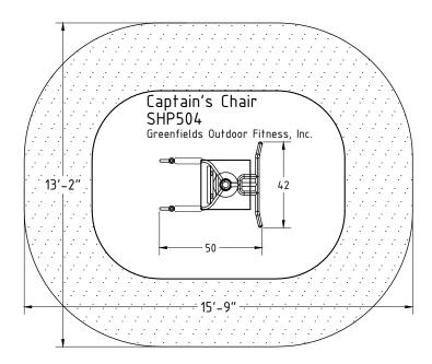
\*Maximum critical fall height (CFH) is defined as the distance between the designated use surface and the surface beneath it.
